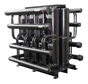
Primary water manifolds are fabricated from 90/10 cupro nickel tube. The secondary fresh water manifolds are fabricated from copper tube. The heat exchangers are mounted on a fabricated steel base. Lifting points are located on the top of the heat exchanger assembly.
