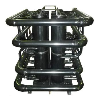
The heat exchanger manifolds are arranged to provide counter flow between the primary and secondary fluid circuits and reverse return to maintain balance pressure drop across the heat exchangers.
