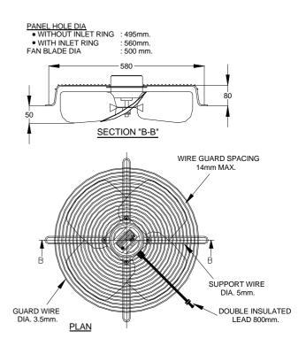
Model PDT-450 (18"). Voltage: 240V 50Hz.
